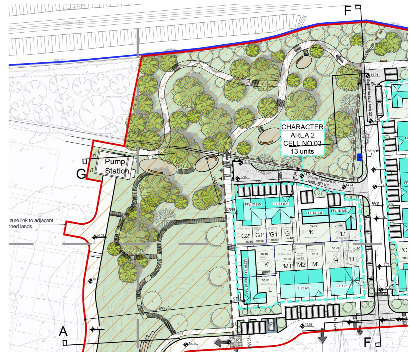
Figure 32. Final submission layout with pumping station outside the tree group.
