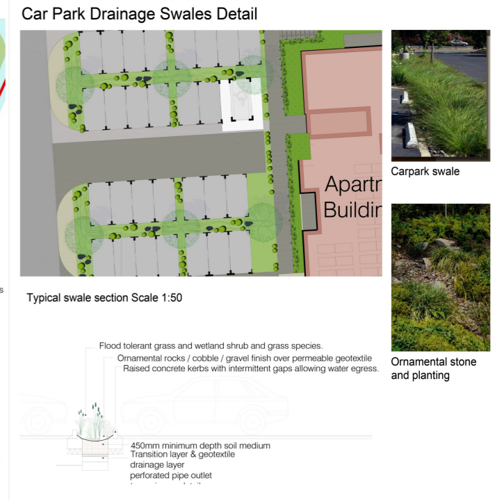
Figure 63. Swale details to carparking areas
